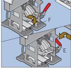
Drop safety latch F and clamp E by pointing the clamp handle towards the seat base
