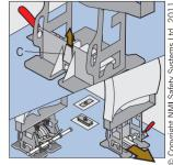
Lift the drop lock C at the back of the seat and slide the seat base forward off the floor
