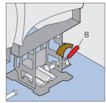
Unclamp wall seat by turning clamp handle B away from the
