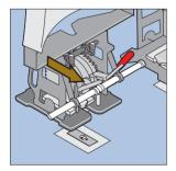
Slide the seat base onto the raised floor pocket
