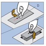
Raise the floor pocket nearest the wall by turning D to align with the dot and then pulling it
