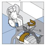
Assist the wheelchair user if necessary to remove their seatbelt. Remove any support cushion. To release the webbing belts rotate safety catch N from back of M. Push M as far as it will go and rotate N so it holds M in up position
