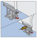
Slide wall seat base onto the raised floor pocket
