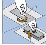
Raise the floor pocket closest to one you just closed by turning D to align with the dot and then pulling it up
