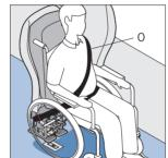
Now assist and apply the inertia belt O located on the seat back around the wheelchair passenger
