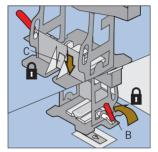
Lower drop lock C and clamp to lock by turning the clamp handle B towards the seat. The side seat is now in the side position
